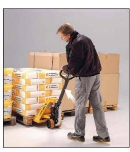
Travel direction is selected by an adjusting handgrip on the handle. Squeeze the handgrip, pump the handle and the truck will be powered in the walking direction. When the handgrip is pressed downward, and the handle is raised, the truck will be powered in the direction of the forks.
